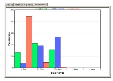
**Range Statistics** provide a comparison of the size and mass distribution of drops on the entire set of slides and in the cloud.
